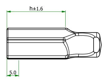
TYPICAL TOLERANCE: THICKNESS 1.0 TO 1.6mm (MEASURED OVER THE FIRST 5mm OF THE MOULDING)
