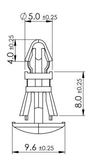
TO SNAP LOCK INTO A Ø4 ±0.08 HOLE, INTO A 1.6 NOM THICK PANEL.
